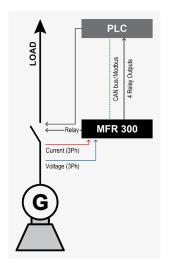
In this generator related application the device is used as a transducer with monitoring functions. The control can be used to open a breaker.
